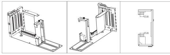
The GPU bracket can be adjusted in length, height and width to support most sizes of GPU cards. Use the silicone pads provided in accessory bag for slim GPU cards.
