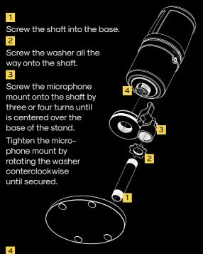
Insert the SVIVE HYDRA MICROPHONE PRO's mounting threads into the microphone mount.
